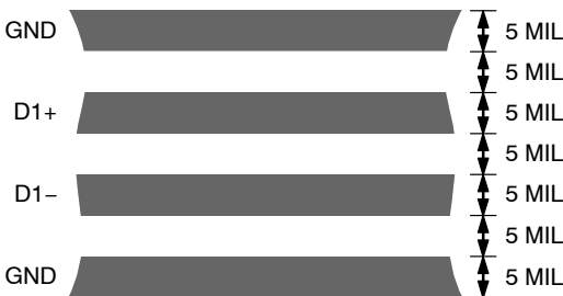
Figure 17. Arrangement of Signal Tracks
