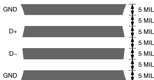
Figure 16. Arrangement of Signal Tracks
