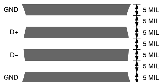
Figure 16. Arrangement of Signal Tracks
