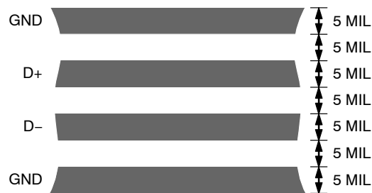
Figure 22. Typical Arrangement of Signal Tracks
