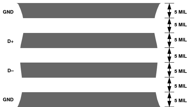
Figure 22. Typical Arrangement of Signal Tracks
