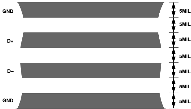
Figure 16. Typical Arrangement of Signal Tracks
