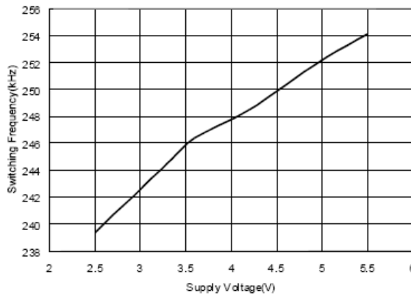
17. Switching Frequency VS Supply Voltage
