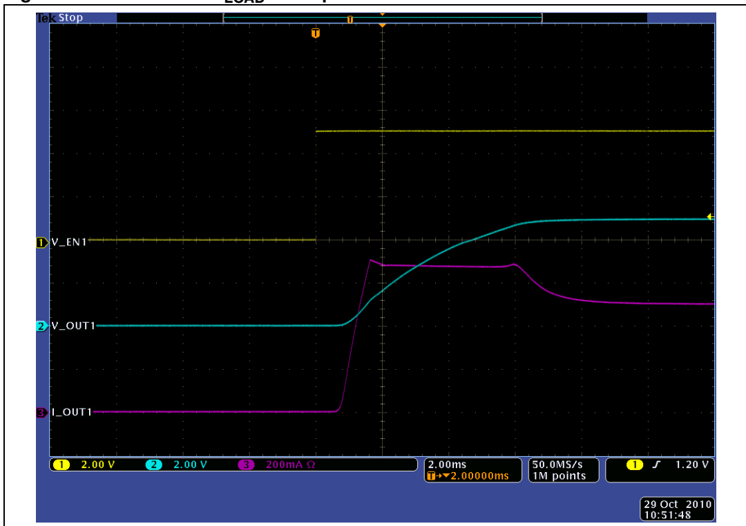
Figure 11. Turn-on for C_{LOAD} = 470 \mu F
