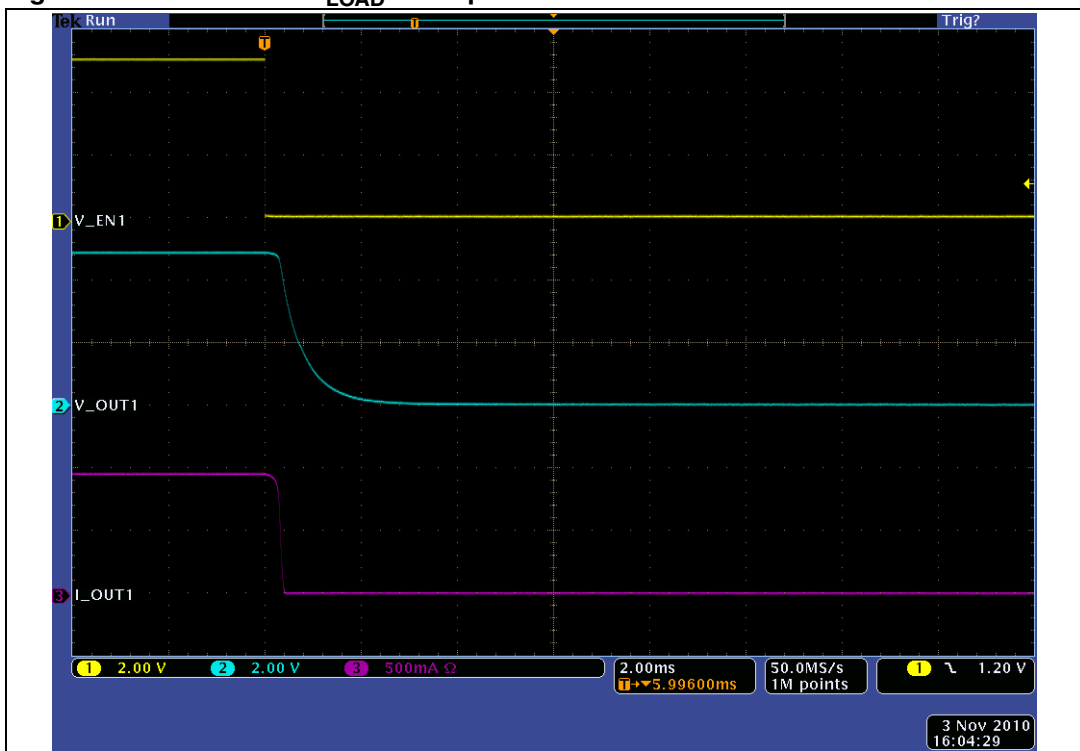
Figure 33. Turn-off for C_{LOAD} = 100 \mu F
