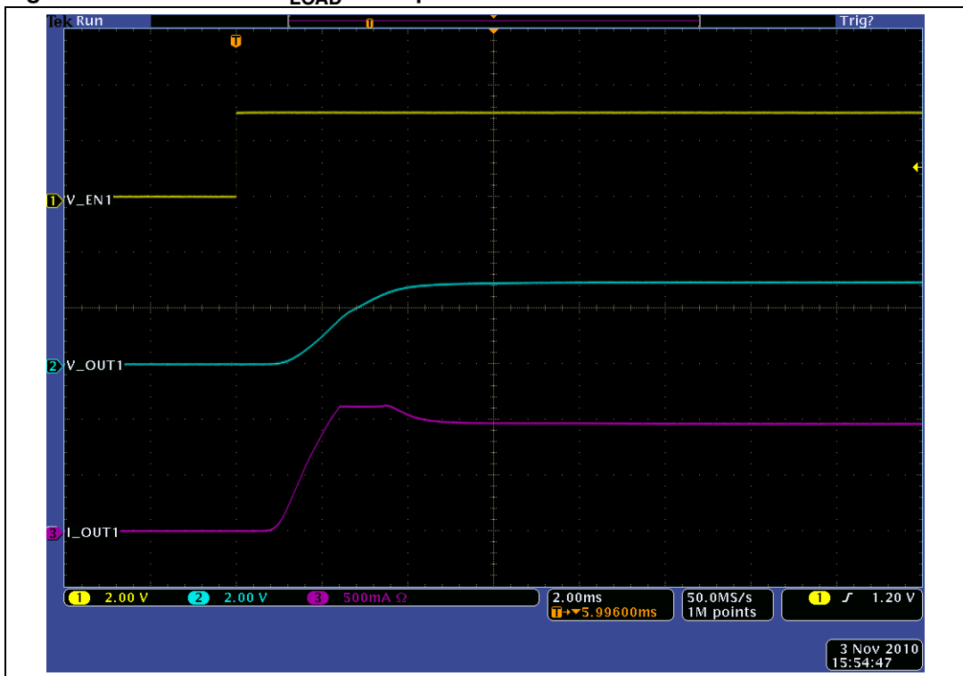
Figure 25. Turn-on for C_{LOAD} = 470 \mu F
