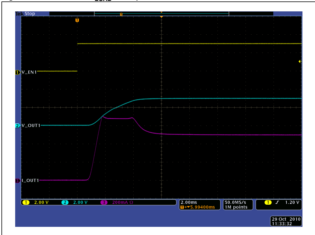
Figure 5. Turn-on for C_{LOAD} = 470 \mu F
