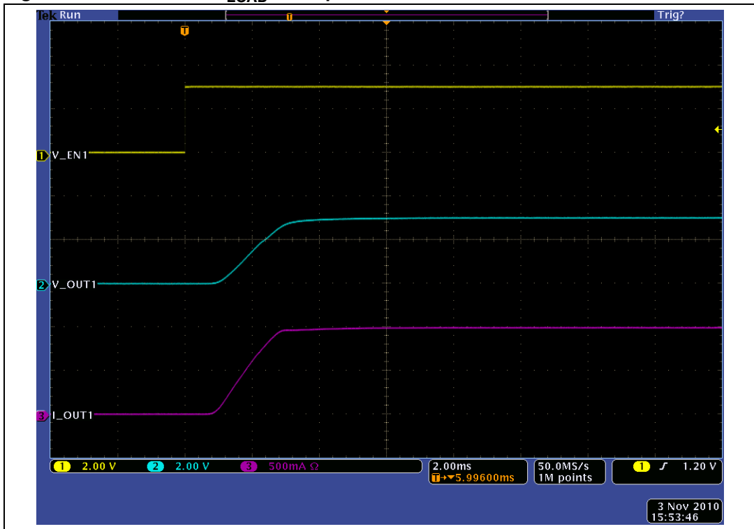
Figure 25. Turn-on for C_{LOAD} = 470 \mu F
