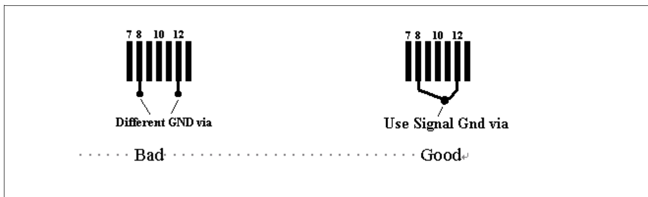
Figure 15 Connection of pin12(GndRef) and pin8(GndR)
