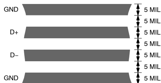
Figure 28. Arrangement of Signal Tracks
