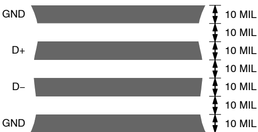
Figure 18. Typical Arrangement of Signal Tracks
