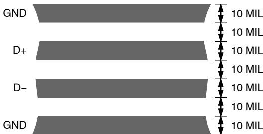
Figure 19. Arrangement of Signal Tracks
