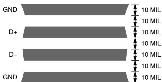
Figure 19. Arrangement of Signal Tracks
