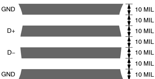
Figure 19. Arrangement of Signal Tracks
