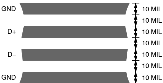
Figure 19. Arrangement of Signal Tracks
