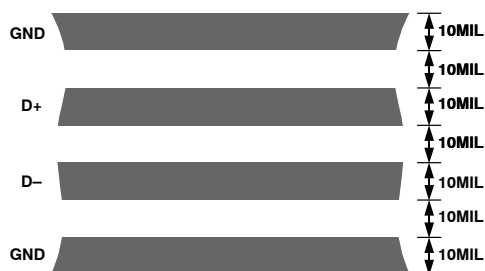
Figure 34. Arrangement of Signal Tracks
