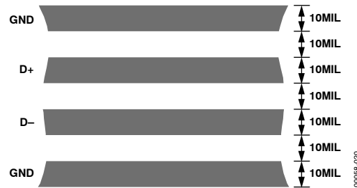
Figure 20. Arrangement of Signal Tracks
