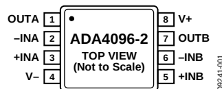
Figure 1. 8-Lead, MSOP (RM-8), ADA4096-2
