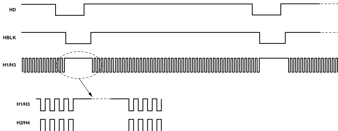
Figure 24. Horizontal Blanking (HBLK) Pulse Placement
