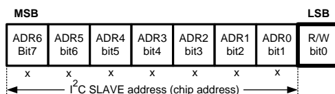
Figure 23. I 2 C Chip Address
