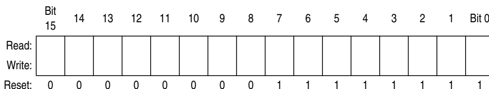
Figure 4-4. Stack Pointer (SP)
