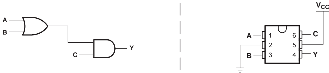
Figure 3. Y = (A + B) \bullet C
