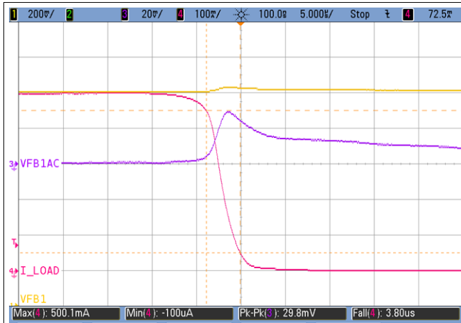
VCC1 = 3.8 V Vout = 1.2 V PWM Mode Figure 7-2. VDD1 Falling Load Transient Response
