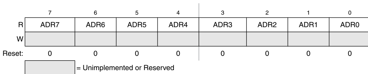
Figure 14-7. Data Result Low Register (ADC1RL)
