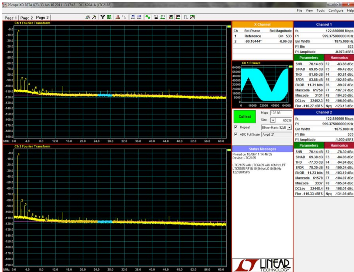
Figure 37. f_{RF} = 845\text{MHz} Receiver Noise Floor Test, f_{LO} = 846\text{MHz} . Ch.1 Is the I-Channel and Ch.2 Is the Q-Channel. Tested without LNA
