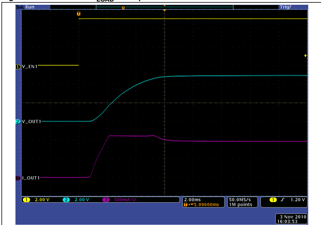
Figure 31. Turn-on for C_{LOAD} = 470 \mu F
