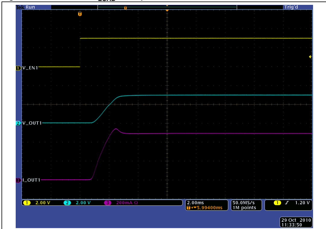
Figure 5. Turn-on for C_{LOAD} = 470 \mu F
