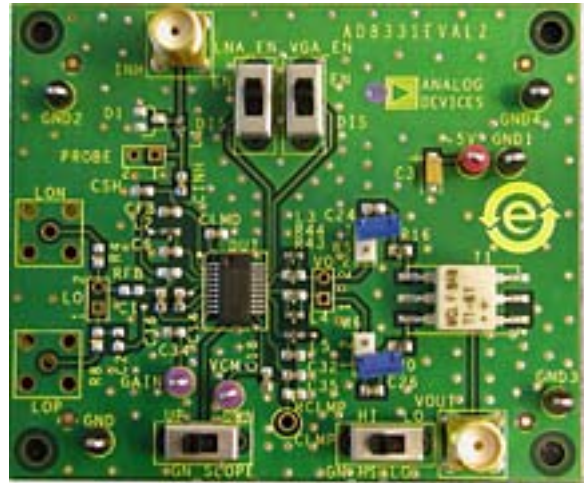
Figure 95. Photograph of AD8331-EVALZ
