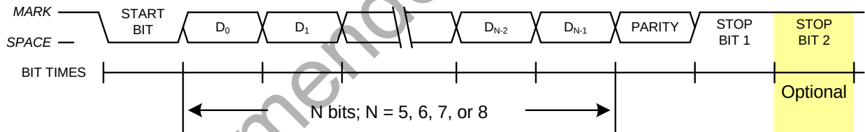
Figure 26.3. UART1 Timing With Parity
