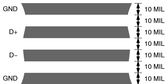
Figure 19. Arrangement of Signal Tracks
