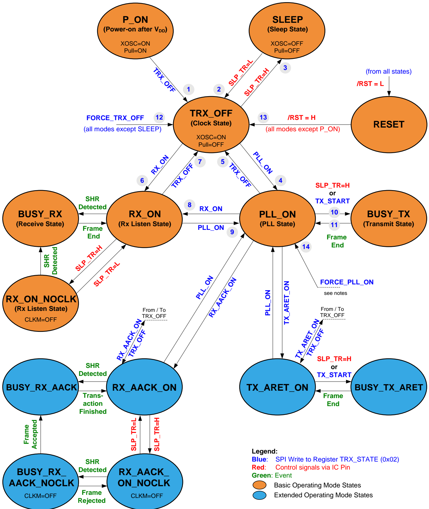
Figure 7-10. Extended Operating Mode State Diagram.
