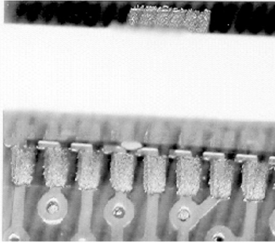
Picture 1. Castellations misaligned to land pads in X-axis before reflow.
