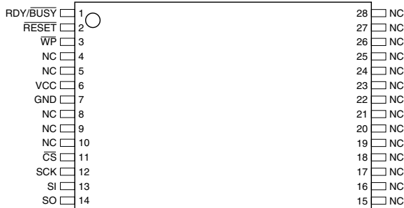
Figure 2-1. TSOP Top View – Type 1
