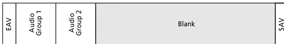
Correct placement of Ancillary Data within HANC Space
