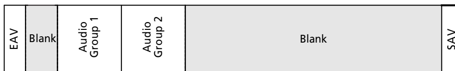
HANC with space between EAV and Ancillary Data (Audio Packets will be deleted)
