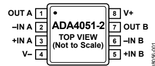
Figure 3. 8-Lead MSOP (RM-8)
