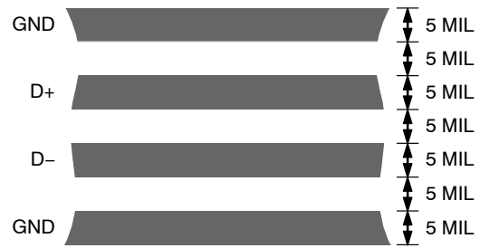
Figure 22. Typical Arrangement of Signal Tracks
