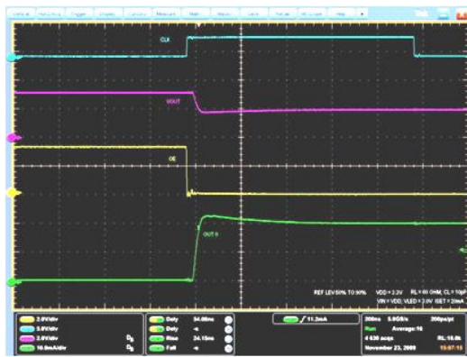
Figure 20: Turn ON output current characteristics (1)
