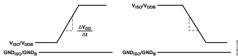
Figure 21. Transient Immunity Waveforms, Output Supplies
