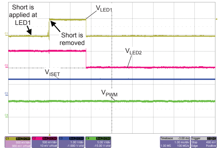
Figure 6: One LED is Shorted to GND. The IC will not proceed with power up until LED pin is released, at which point the LED is checked to see if it used.
