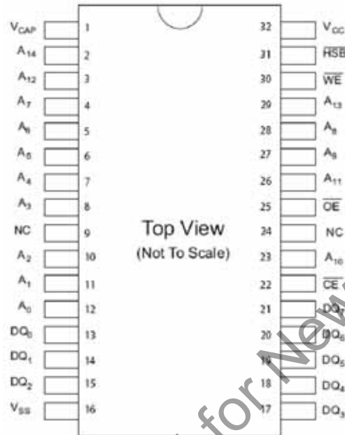
Figure 1. Pin Diagram - 32-Pin SOIC/32-Pin PDIP
