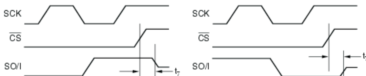
Figure 11. High Impedance Output Timing Diagram
