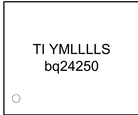
YFF Package Symbol (Top Side Symbol for bq2425x)
