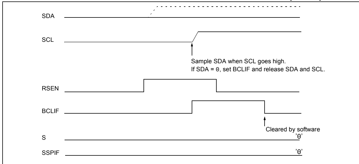
FIGURE 16-36: BUS COLLISION DURING A REPEATED START CONDITION (CASE 1)
