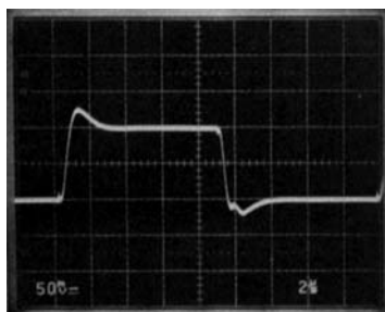
Small-Signal Transient Response, Pin 1 = V -
