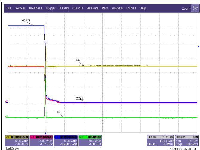
Figure 28. Hot Short on Output with No Load (zoomed out)
