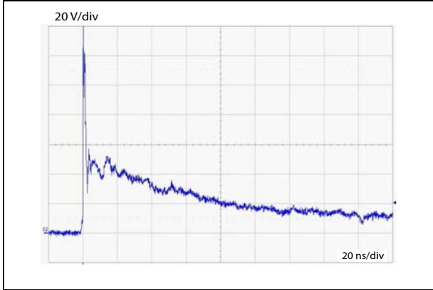
Figure 7. ESD response to ISO 10605, C = 150 pF, R = 330 Ω (+8 kV contact)
