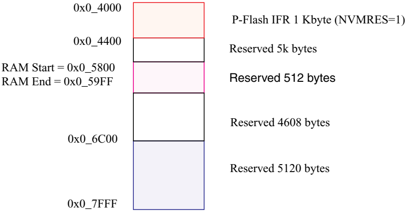
Figure 27-3. Memory Controller Resource Memory Map (NVMRES=1)
