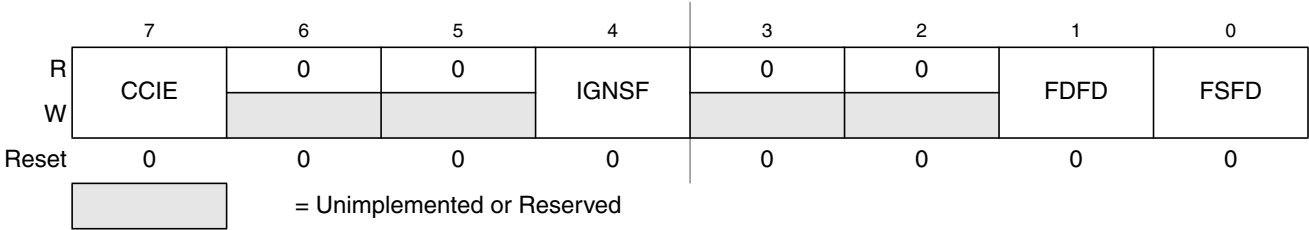
Figure 25-9. Flash Configuration Register (FCNFG)
