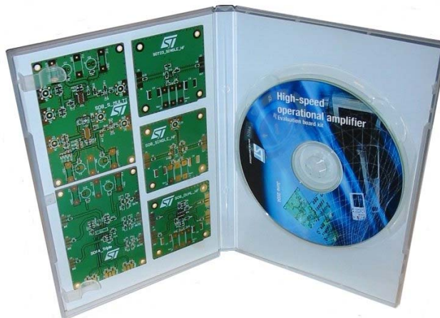
Figure 44. Evaluation kit for high-speed op-amps
