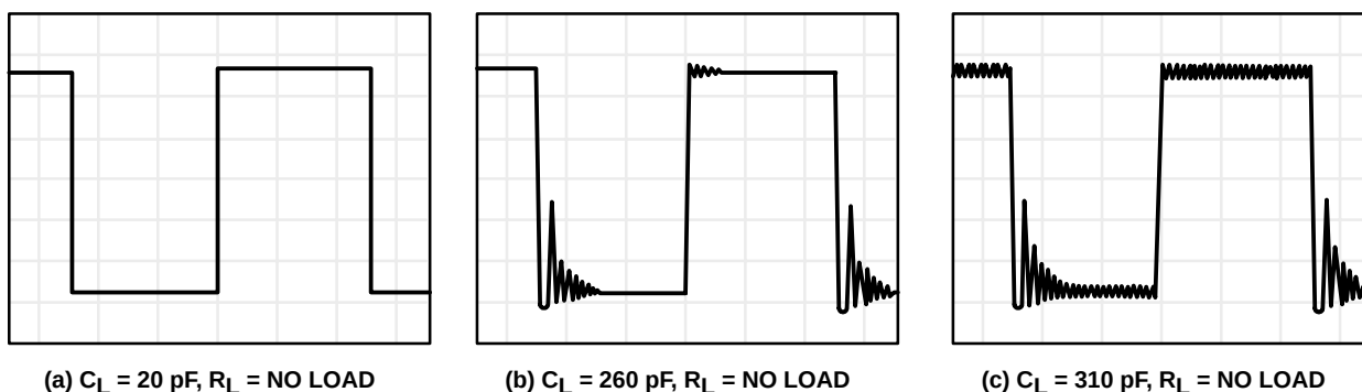
Figure 112. Effect of Capacitive Loads in Low-Bias Mode
