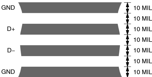
Figure 19. Arrangement of Signal Tracks
