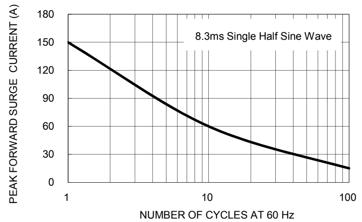
FIG. 2 MAXIMUM NON-REPETITIVE FORWARD SURGE CURRENT PER LEG
